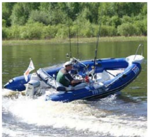
**Inflatable boat with rigid glass reinforced plastic hull (RIB)**
